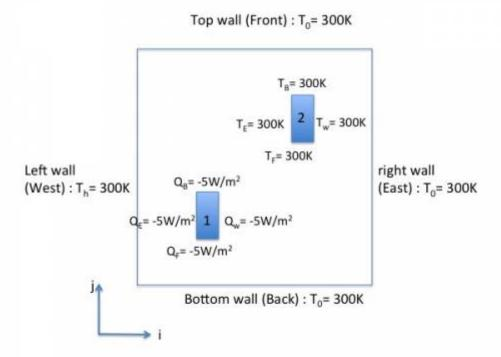
We need two **WBCT** for setting the two different sets of wall boundary conditions, the first one for the imposed temperature, the second one for the imposed heat flux. We also need to set two **IBD** in order to define the positions of the couple of bars.
