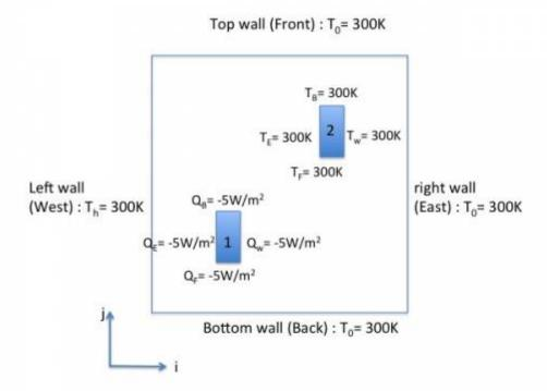
We need to two **WBCP** for setting the two different sets of wall boundary conditions, the first one for the imposed temperature, the second one for the imposed heat flux. We also need to state two **IBD** in order to define the positions of the couple of bars.
