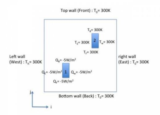
We need to two **WBCT** for setting the two different sets of wall boundary conditions, the first one for the imposed temperature, the second one for the imposed heat flux. We also need to state two **IBD** in order to define the positions of the couple of bars.
