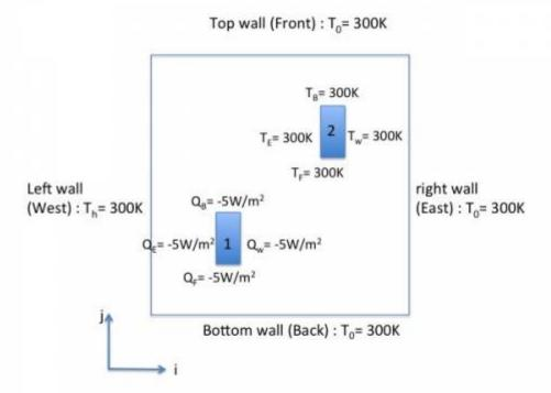
We need to two **WBCT** for setting the two different sets of wall boundary conditions, the first one for the imposed temperature, the second one for the imposed heat flux. We also need to state two **IBD** in order to define the positions of the couple of bars.
