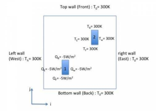
We need to two **WBCT** for setting the two different sets of wall boundary conditions, the first one for the imposed temperature, the second one for the imposed heat flux. We also need to set two **IBD** in order to define the positions of the couple of bars.
